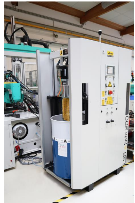
Photo 2: The injection moulding machine in the RICO training workshop was equipped with the latest dosing technology from Reinhardt-Technik.
